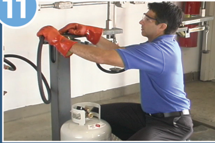
Check the weight of the filled cylinder after the filling connector has been disconnected. If overfilled, bleed off excess propane in a safe location.
