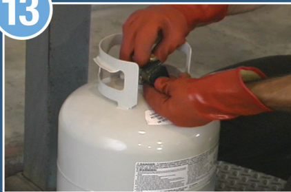
For cylinders 45 lb or less, install a protective cap on a QCC valve or a POL plug if the cylinder is equipped with a POL service valve.
