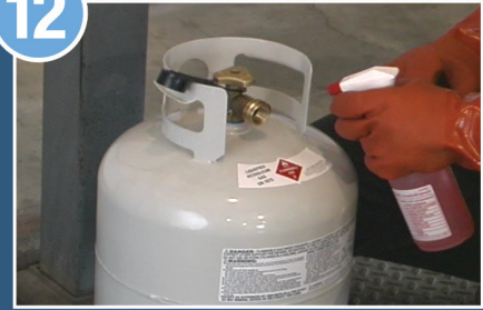
Check the container valves for leaks.
